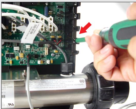
– Remove 1 screw to open the cable holder.
